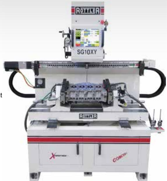
valve seat cutting such as valve seat housing counterboring and valve guide reaming, the spindle is required to be locked vertically. The ACTIV spindle has a pneumatic locking system that locks the spindle sphere rigidly vertically for other types of machining requirements.
